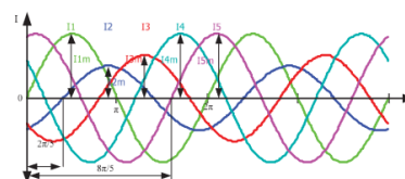
FIGURE 4. Currents generated by a five-phase current source.
